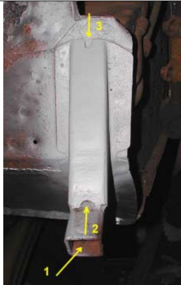
If the front fenders are off, 1 is the same procedure than the previous photo, 2 and 3 can be sprayed with a can. If you have a compressor, blow air in 1, 2 and 3. Wear eye protection!
