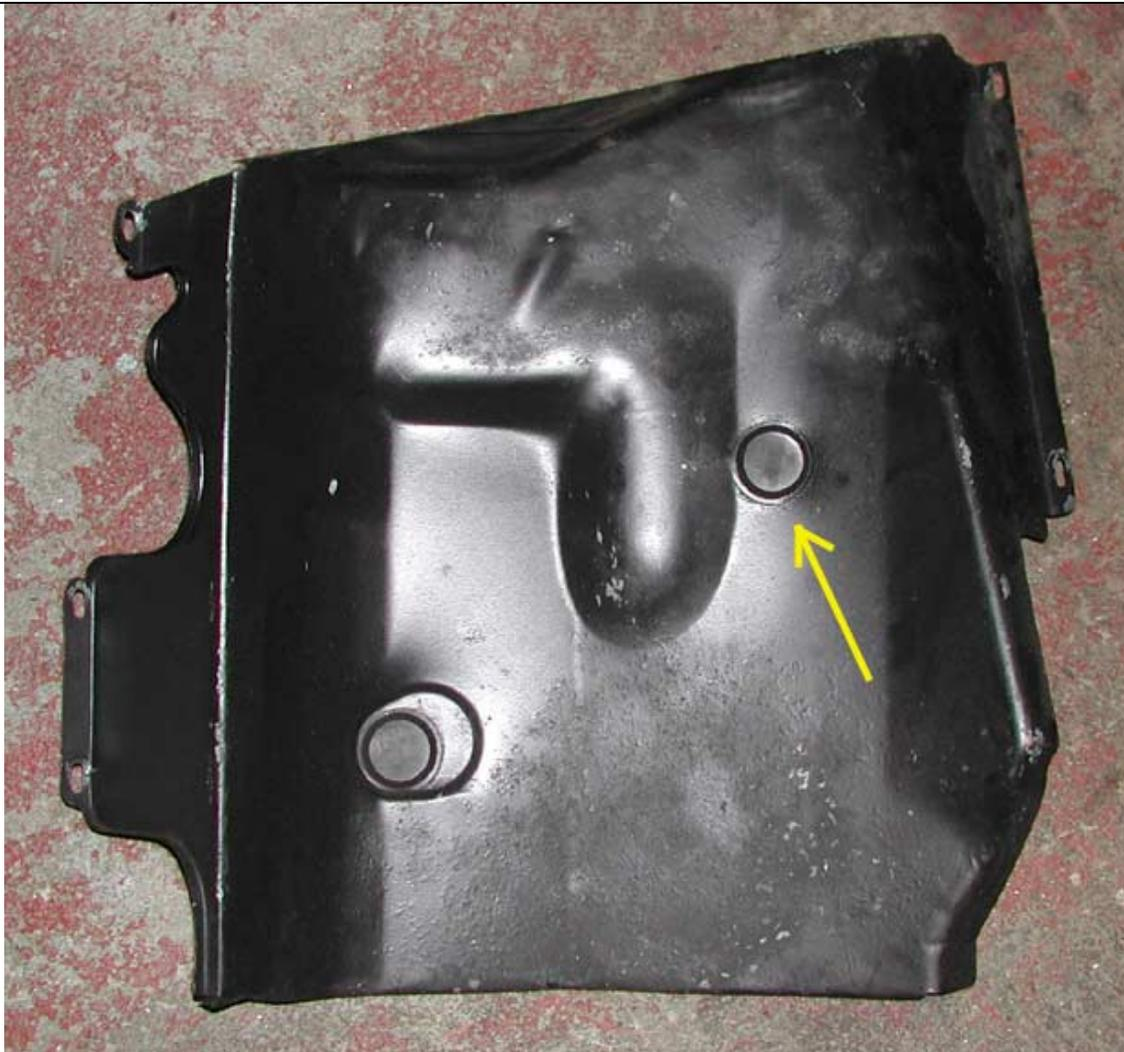
On second and third front, use the grease nipple access holes and spray.
