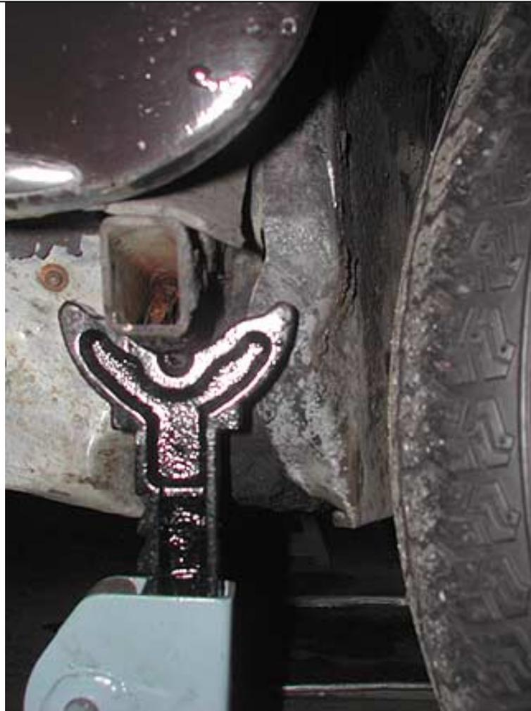
Clean cavity first. If you have a compressor, blow air in cavity. Wear eye protection! Then spray inside.
