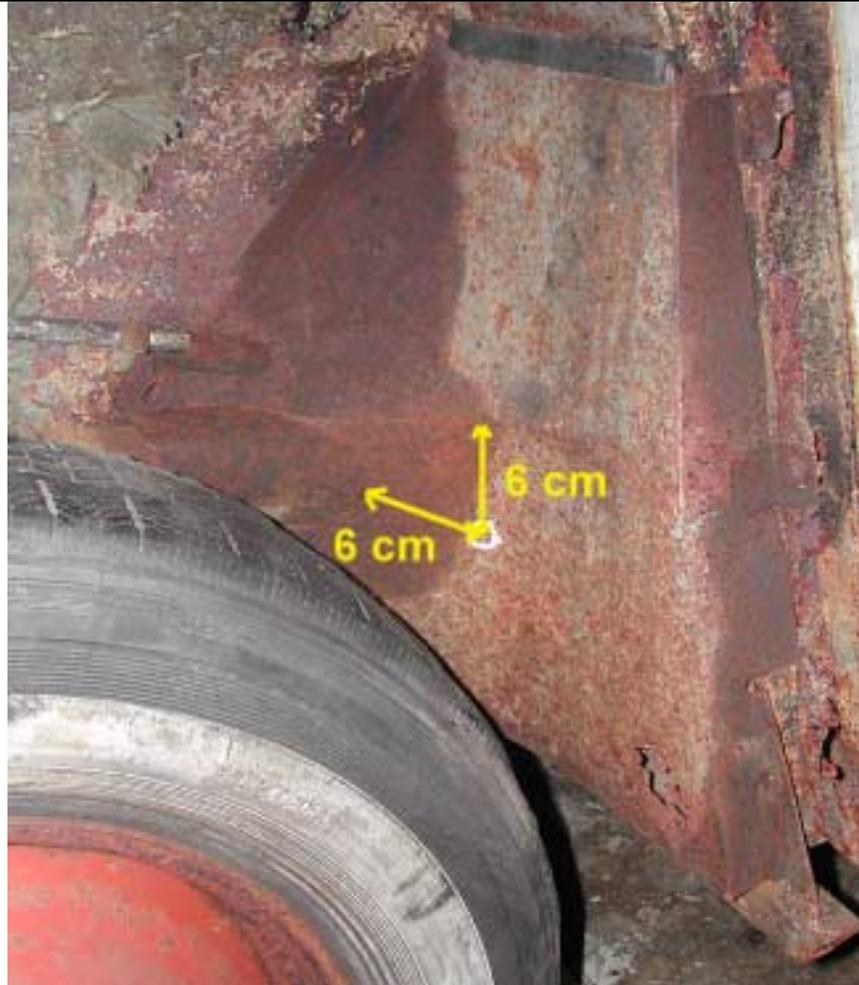
Right side. Drill at 6 cm below the notch. This will give you access to the fuel filler conduit.
