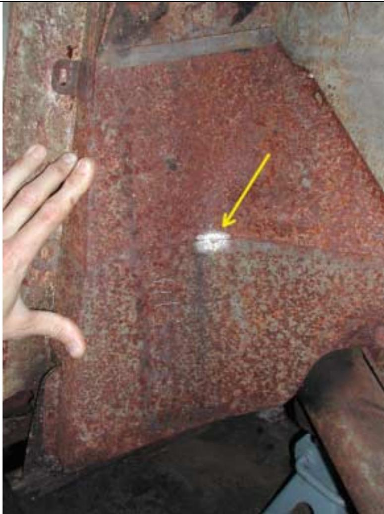
Left side. Drill at the notch. This will give you access to the rear height corrector and linkage.
