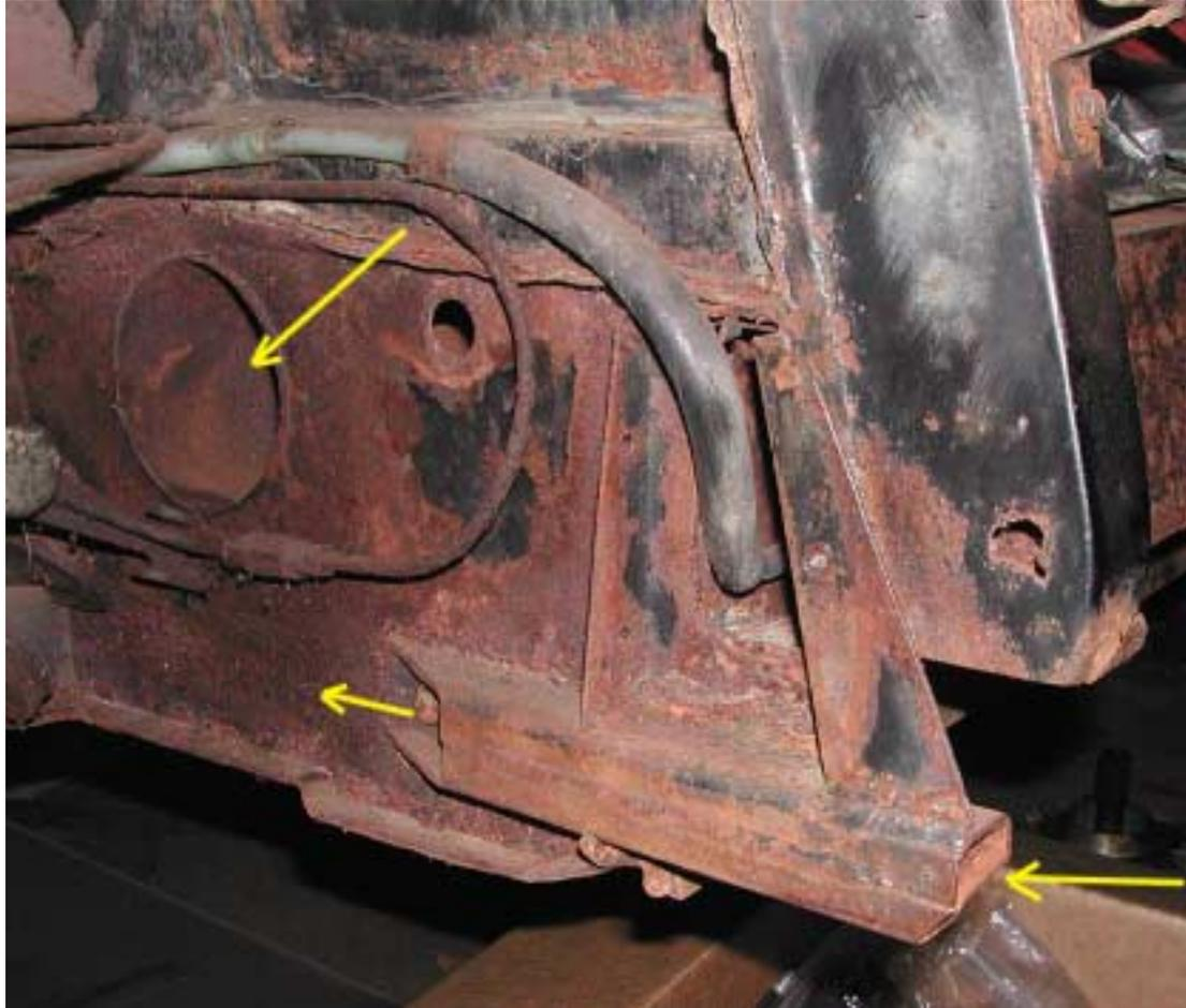
On first front models, clean rear jacking tubes and spray (they are open at the end). To access fuel filler conduit, see oiling point number 13.
