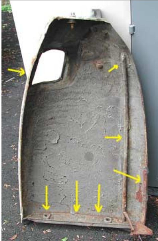
On first models, the fold is on top of the fender (left arrow), on later models, the fold is inside. Spray everywhere water or dirt could seep in
