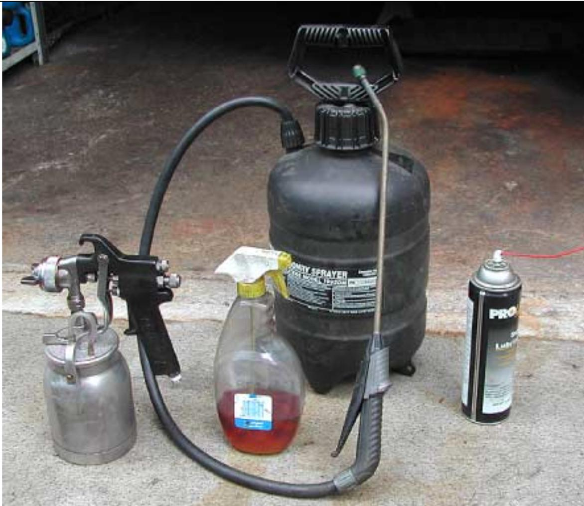
Alternate tools: spray gun for engines and large areas. Without a compressor, you can use a household sprayer, a masonry sprayer and a spray can for small holes.
