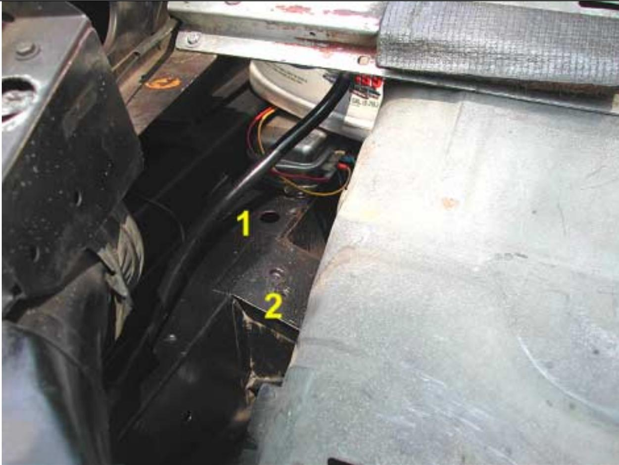
Spray in existing hole (1). Drill 2, spray and plug.
