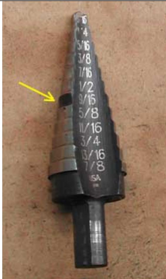
Step drill bit. Use a marker (or masking tape) on the 9/16" step to make sure you do not drill a hole bigger than 1/2"
