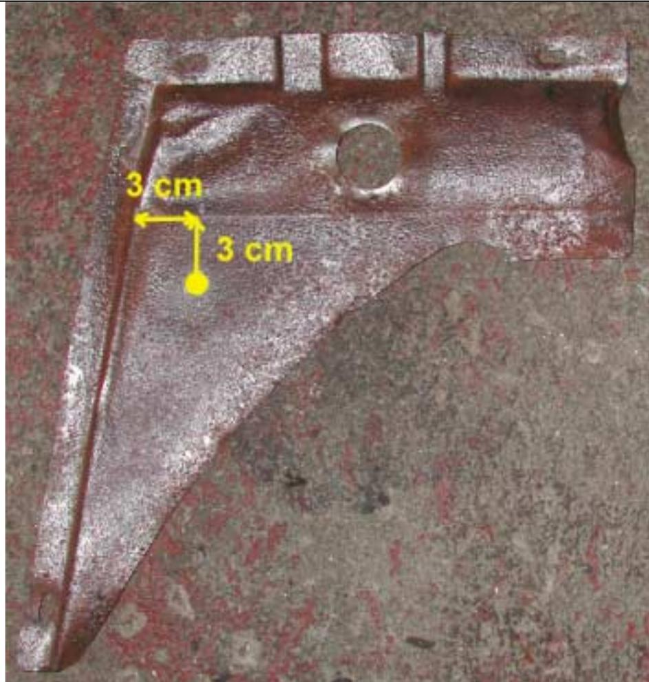
On first front, measure 3 cm from the groove, then 3 cm down with a 90° angle. Drill, spray and plug. This will give you access to sway bar area and corrector on the front.
