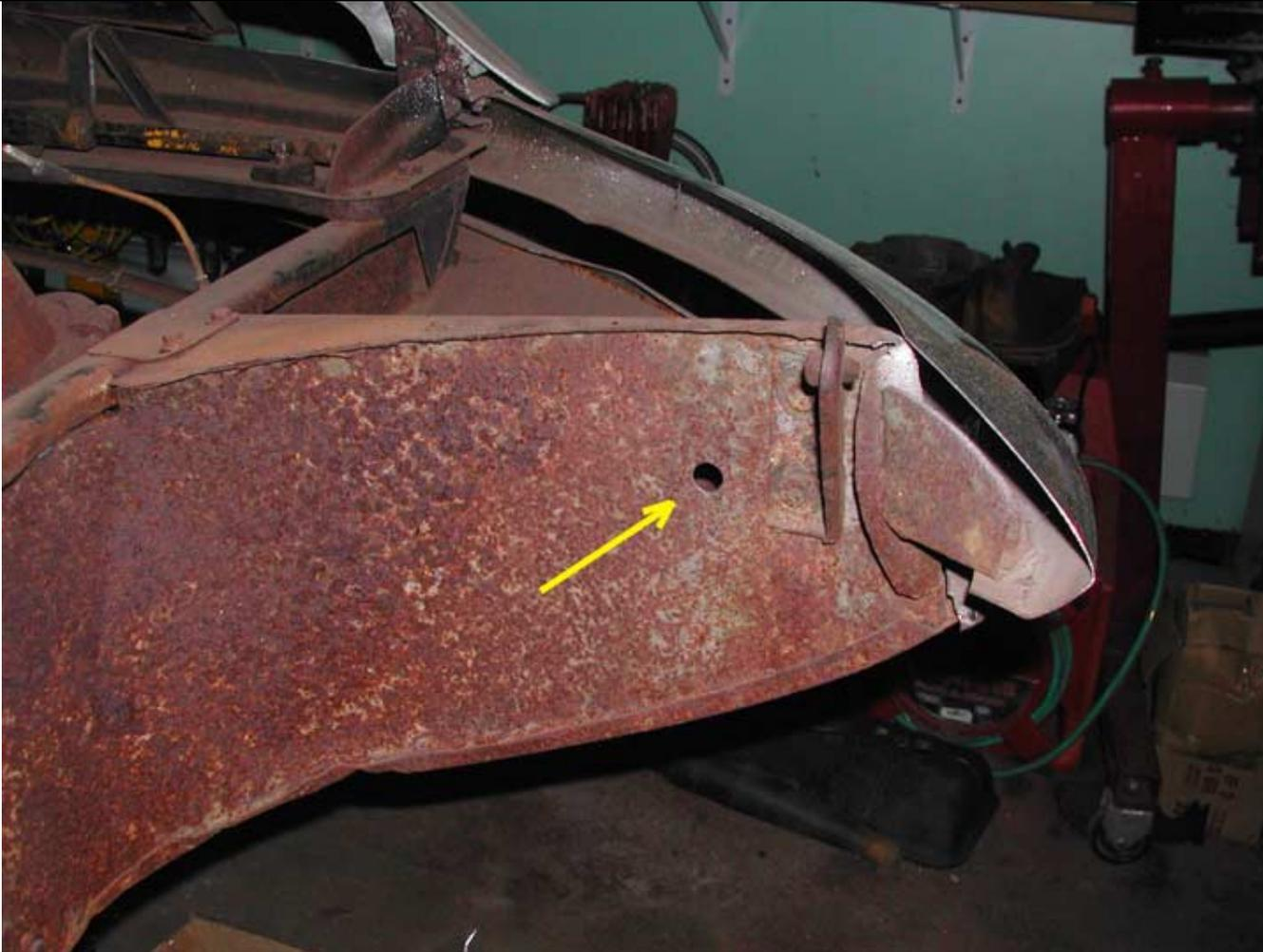
On first front models, drill to be able to spray with the wheel on and turned to the opposite side.
