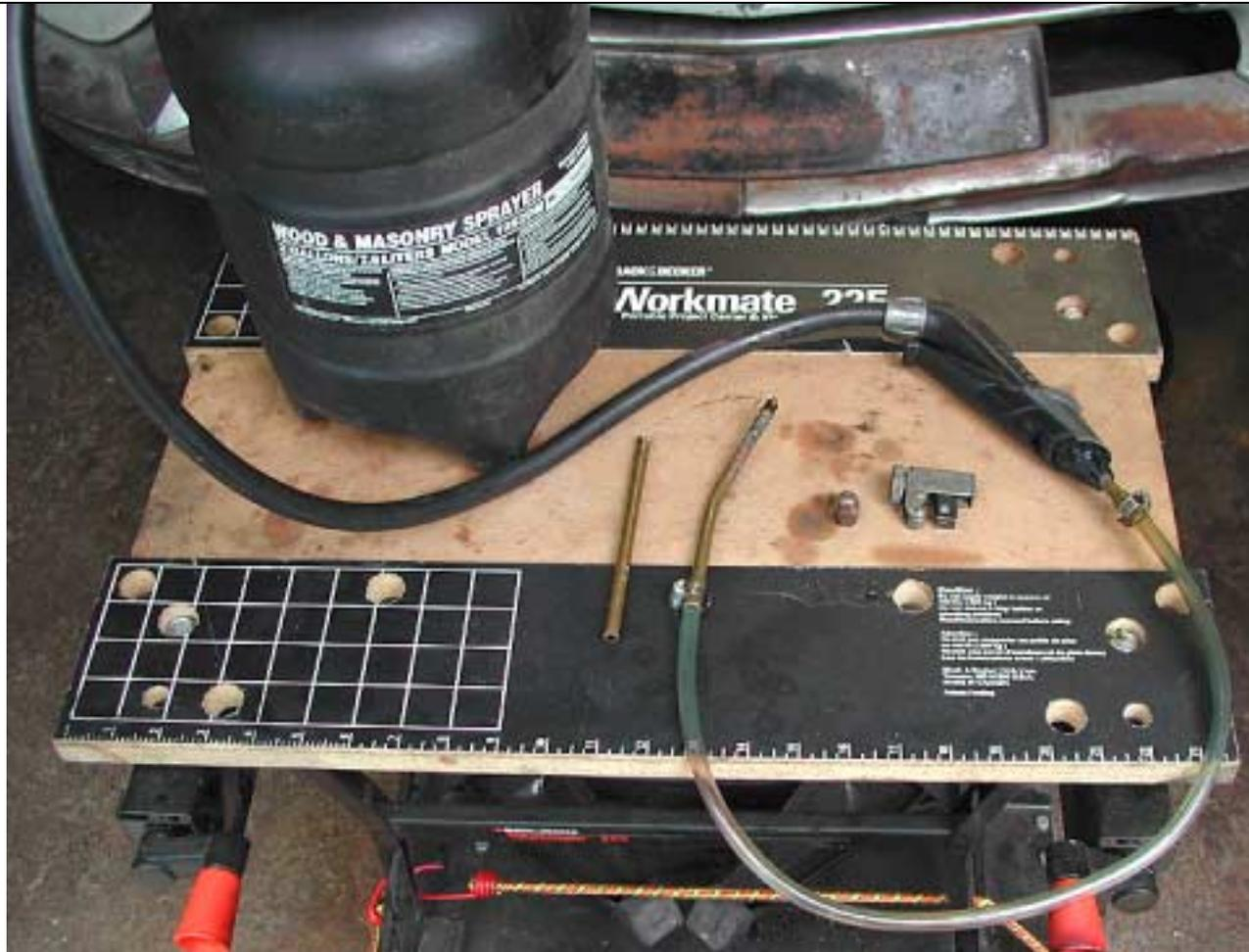
Sprayer after modification. Remove end (due to size), flatten hole and re-drill with 1/16" or smaller. This can shoot over 18'. By turning the tank upside down, this will mix air with the oil, which will make a fine mist.
