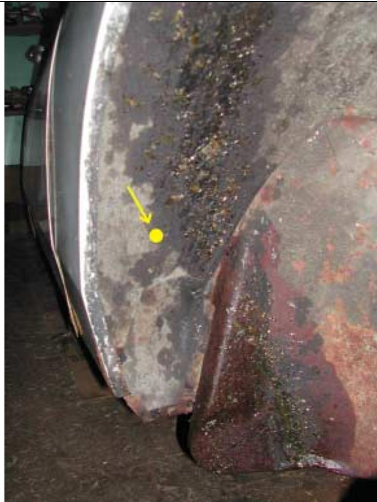
There is an enclosed area in the front fender. You can drill there in order to be able to spray by turning the wheel to this side (right side shown).
