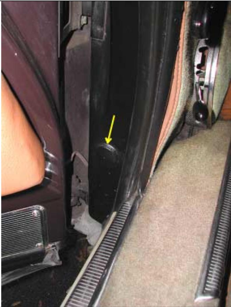
Remove plug and spray in fender guide.
