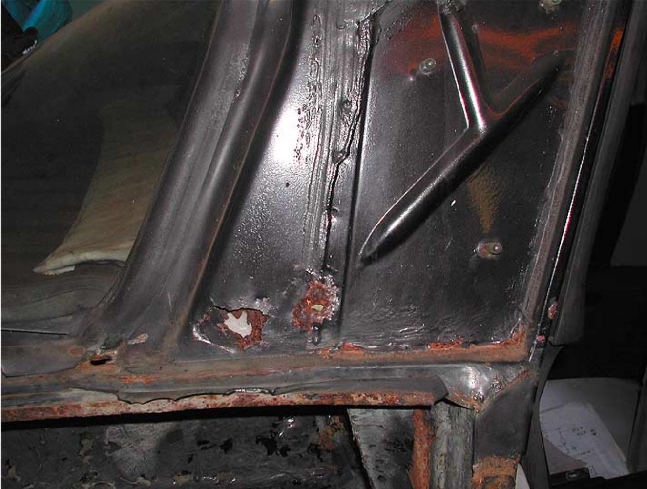
You can treat the C pillar by removing the rear seats and headrests. Do not drill with a step bit due to the lack of clearance between the two steel plates.
