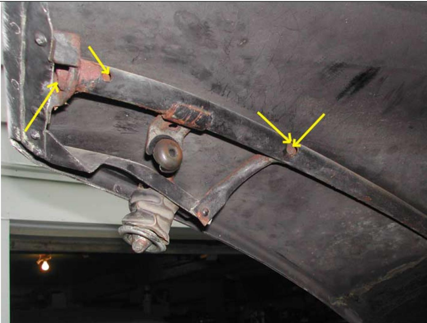
Second front shown. Using a spray can, spray every hole in all directions.
