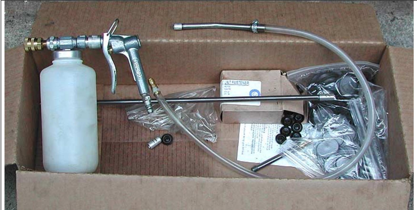
This kit comes with 3 different spray hoses and endings: straight forward, 90 degree angle and backward. The 1/2" plugs can be purchased at your local body shop supplier. A compressor is required to use this kit.
