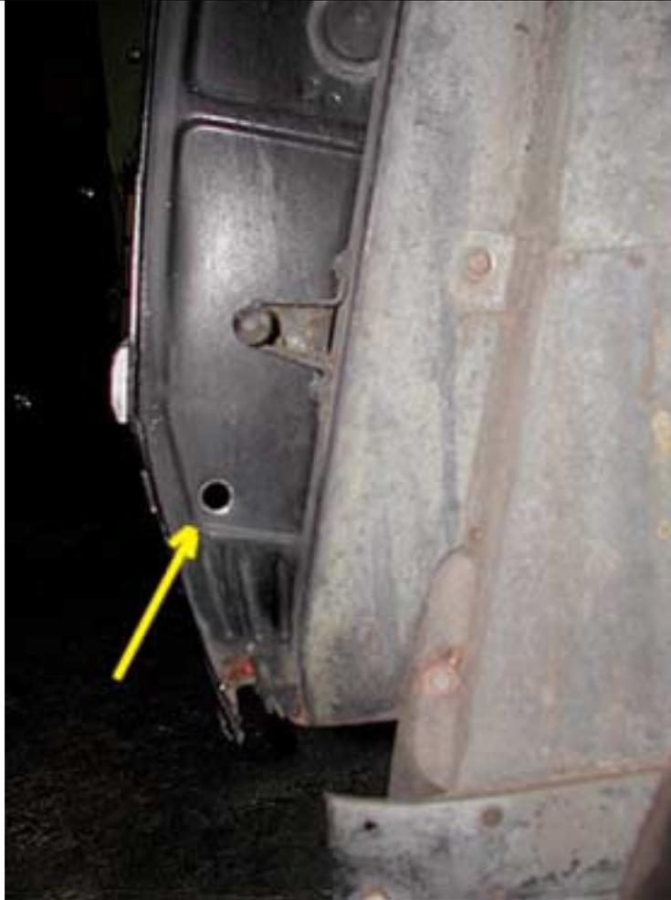
Do not drill in the middle of the door, you will find the railing for the widow. Close the door and drill where indicated.
