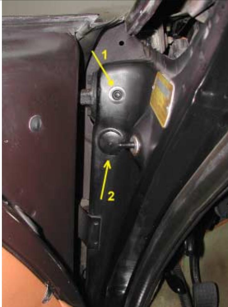
Drill at number one, spray straight and down. Remove plug (2) and spray in fender guide.
