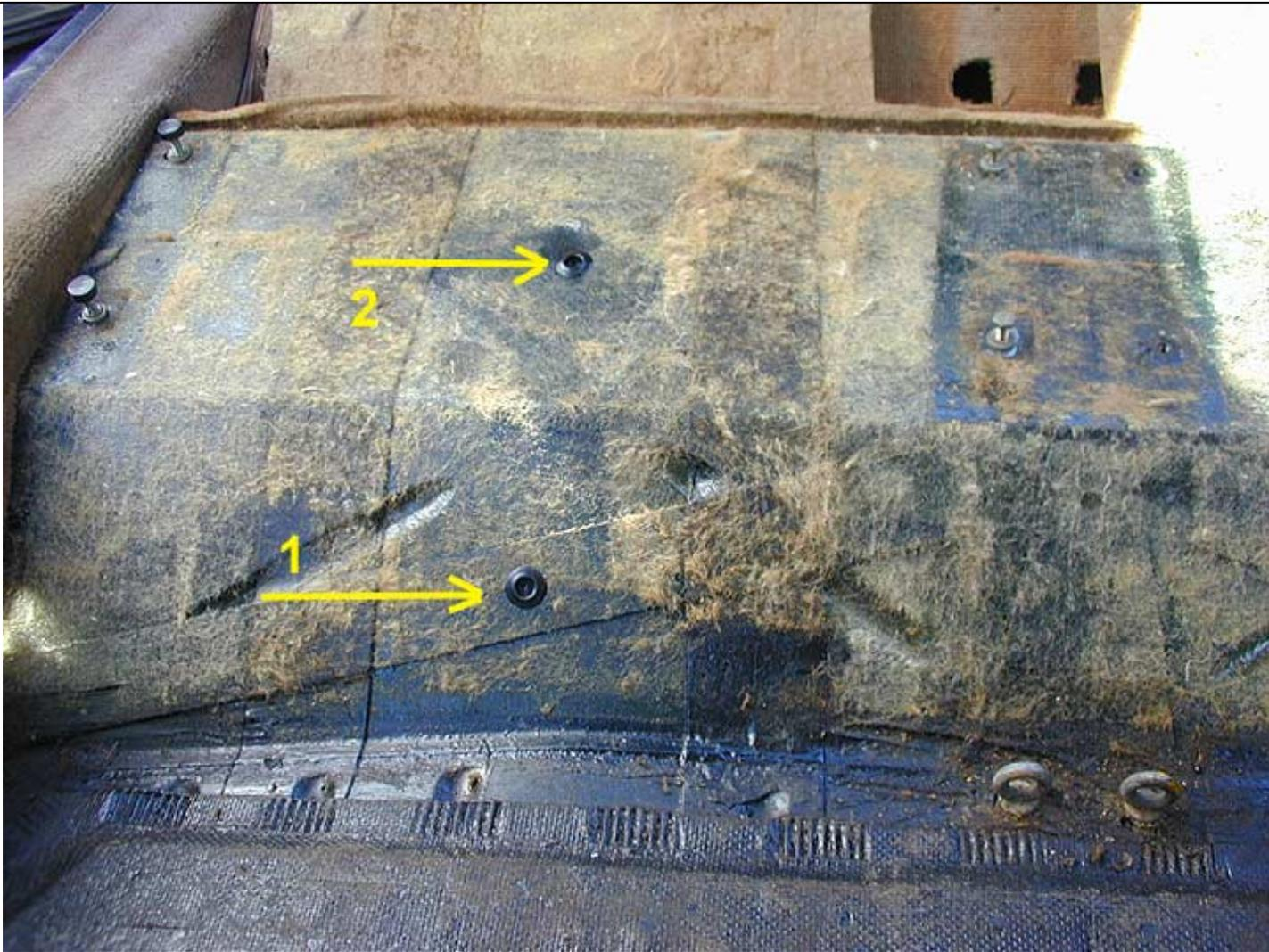
In case the front seats are removed, you can add a second oiling hole (2).
