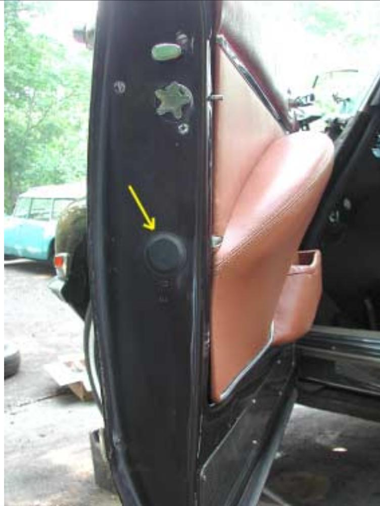
Existing plug. Aim towards the bottom of the door and spray. Keep window up.
