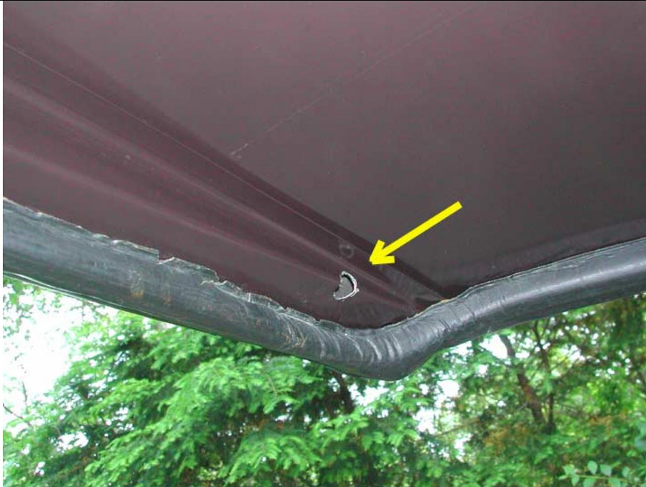
Use existing hole and drill PARALLEL to the trunk lid. The oil will be leaking from the edge of the lid for a while, but this is a very important oiling point.
