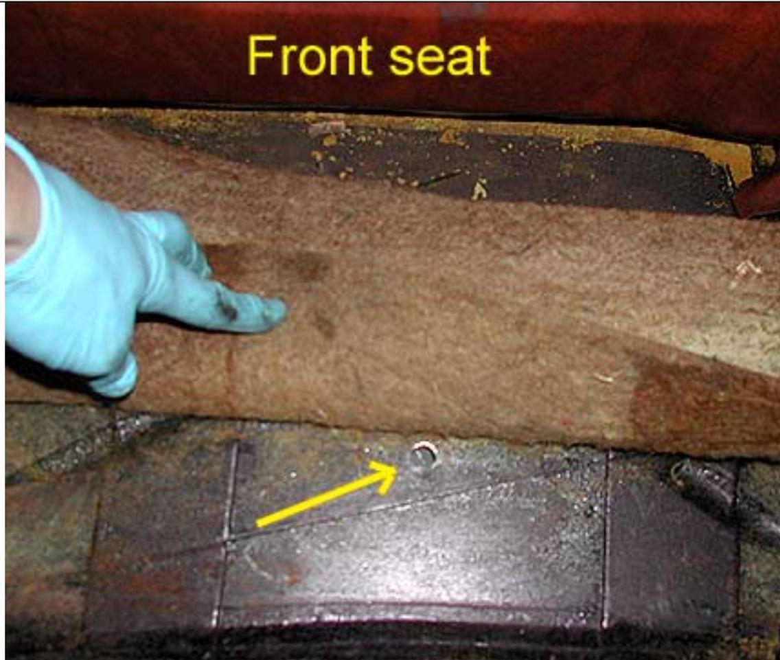
Use a step drill bit on first front cars. Use a regular 1/2" bit on second and third front do to the lack of clearance between the two steel plates. Push front seats towards the front of the vehicle and remove carpet.
